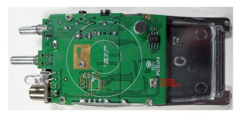
Figure 4 - BF888S disassembled enough to allow the frequency to be adjusted
