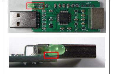
Insert the LED array into the PC board. Ensure it is vertically at right angles to the PC board and parallel to the board edges. Solder the pin farthest from the board end and then recheck the alignment. Adjust as necessary and then solder the remaining pins. Trim excess lead length after soldering.
