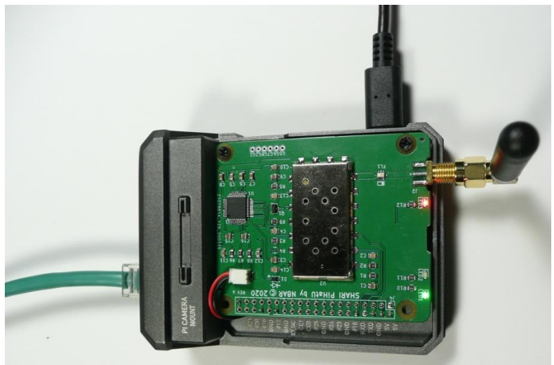
Figure 2 – SHARI PiHatU board installed in case with Raspberry Pi 4
