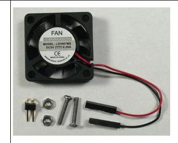
Remove the 2 plastic crimp housings from the female pins on the red and black wires by gently lifting the tab retaining the pin and pulling on the wire. Here is a link to a YouTube video on pin removal.
