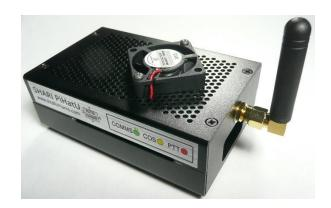
2. <u>Straight 4" Rod Antenna</u> - A vertical mounted SMA antenna jack exits through a hole in the top cover. The kit is supplied with the hole punched in the case top cover. The cooling fan option can still be used with the vertical antenna option.
