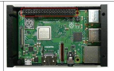
Solder the 40 pins of the GPIO connector.
