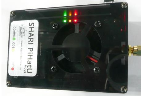
Unlike our other SHARI products that use an SMA connector soldered to the PC board, a coax cable with an SMA connector on one end and a U.FL (IPEX) male connector on the other is used to route the RF signal to the antenna. This simplifies construction and permits the antenna location to be easily changed by the builder.
