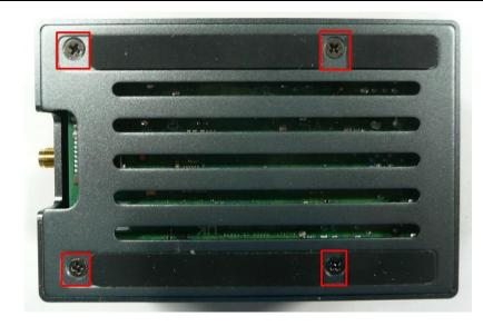
Route the coax cable with SMA connector as shown. Place the star washer onto the SMA connector with its tangs pointing toward the case. Thread a nut onto the SMA connector and tighten.
