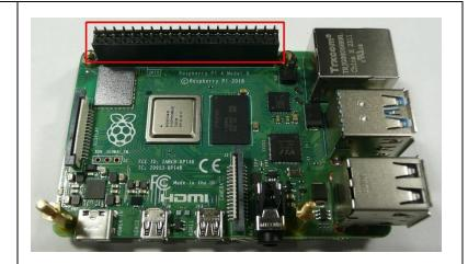
Mount the SHARI PiHat Mod2 PC board onto the GPIO connector pins and the two 11 mm brass standoffs. Install nuts onto the brass standoffs (shown in red boxes). Shift the positions of the two PC boards so that the GPIO connector pins are approximately centered in the PCB holes and tighten the mounting hardware (two nuts and 4 standoffs).
