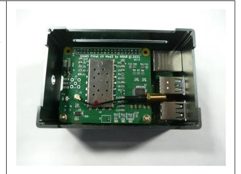
Fasten the PC board assembly in place using the bottom cover and four screws.
