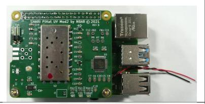
Apply solder to the TP06 and TP10 pads . (outlined in yellow) on the Pi 4B to create a spherical mound of solder on the pad. Solder the end of the black wire to TP06 and the red wire to TP10 by reheating the solder and pushing the end of the wire into the solder. Route the wires as shown and apply hot glue or equivalent (location outlined in red) to act as a strain relief for the wire and hold it in place.
