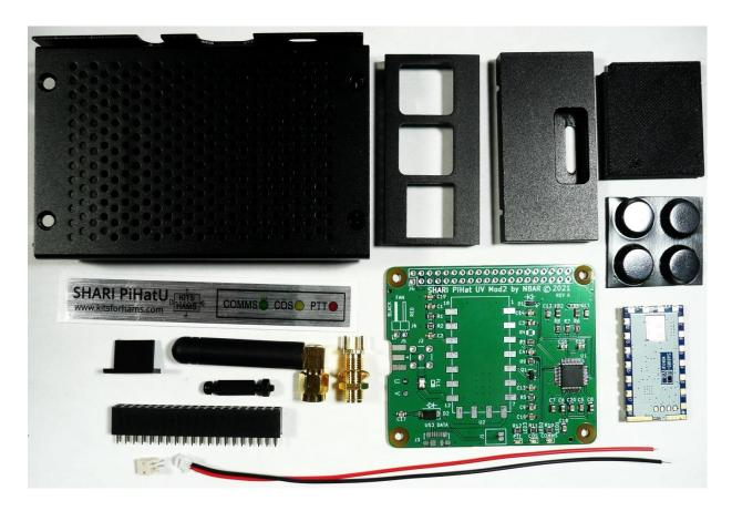
The above photo shows the parts (except ferrite cores) in the kit for the elbow antenna kit option.
