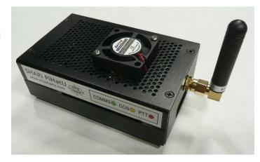
The SHARI PiHat PCB is implemented with surface mount parts, a NiceRF radio module with castellated holes for mounting to the PC board and throughhole connectors. The board is supplied with all the small surface mount parts installed. The kit builder installs two through-hole connectors, an SMA RF connector and the SA818 radio module.
