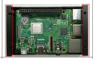
Install the 2 row, 40 position female pin header GPIO connector onto the matching connector on the Pi. Press firmly in place so there is no gap between the connector plastic bodies.
