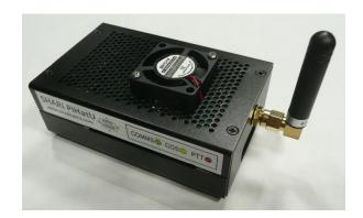
2. <u>Straight 4" Rod Antenna</u> - A vertical mounted SMA antenna jack exits through a hole in the top cover. The kit is supplied with the hole punched in the case top cover. The cooling fan option can still be used with the vertical antenna option.
