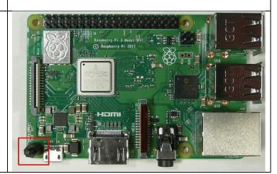
Place the Pi in the bottom half of the Unistorm case and secure with one silver colored Phillips mounting screw.
