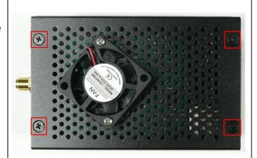
Install four polyurethane feet onto the four corners of the bottom cover.
