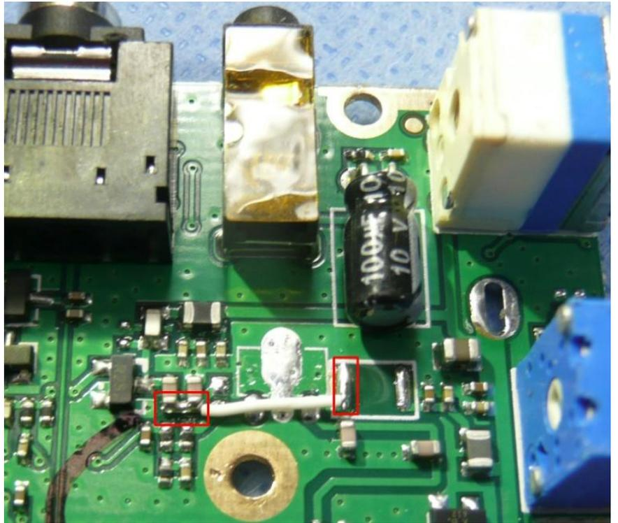
Prepare a 1 ½ inch piece of 30 AWG solid core Teflon wire and solder one end to pin 1 of the IC on the BF-888S board as shown in the photo. While not absolutely necessary, it is suggested that hot glue or silicone RTV be applied to the wire near the edge of the board to provide strain relief to minimize the possibility of the wire breaking at the solder joint.
