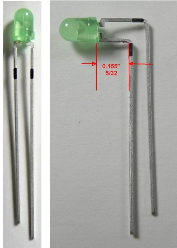
Install a green LED in the LED5 position on the motherboard. The annular ring at the base of the LED should be in contact with the PC board and behind the edge of the board
