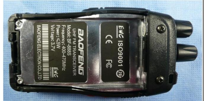
Remove the two plastic control knobs. The longer knob fits tightly. Use a flat bladed screwdriver to pry it off if necessary. Save the knobs for final assembly.
