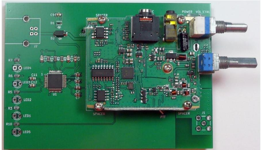
Solder the five wires to the appropriate labeled pads (VOL\_CTRL, POWER, MIC, COS and PTT) on the motherboard by melting a pool of solder on each pad and let it cool. Place the stripped wire onto the solder. Apply the tip of your soldering iron to the wire and push it down into the solder.
