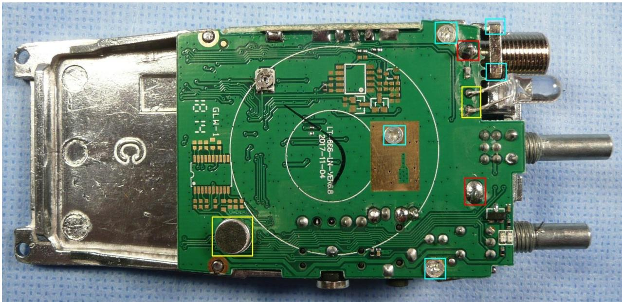
This is the BF-888S PCB assembly with the LED removed, the mic removed, the RF connector removed and the solder removed from the antenna center conductor and DC power connection points.
