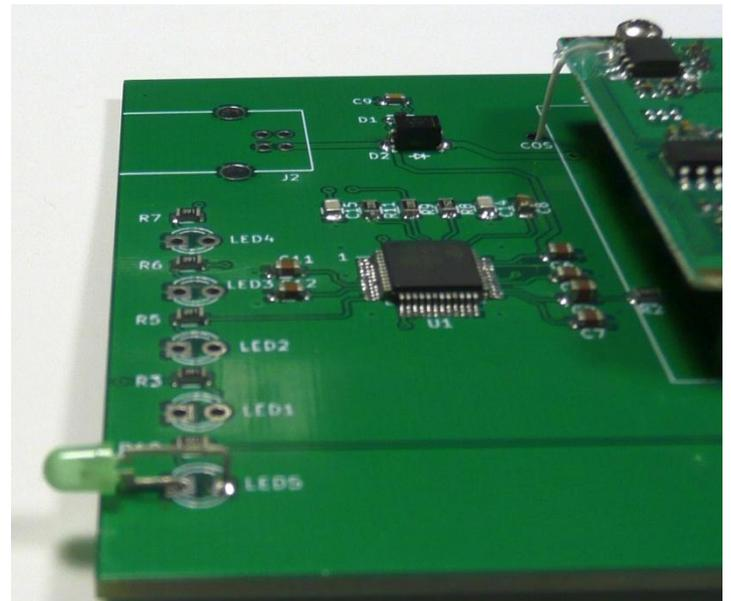
Install the remaining 4 LEDs on the motherboard in the positions shown in the photo. Trim the excess lead length from all five LEDs. Save two of the longer pieces of wire for use in the next paragraph.
