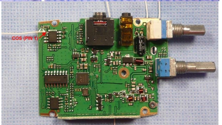
Using solid core 30 AWG Teflon wire, solder four 1 ½" jumper wires to the points on the BF888S board shown in the photo (PTT, MIC, POWER and VOL\_CTRL). While not absolutely necessary, it is suggested that hot glue or silicone RTV be applied to the wire near the edge of the board to provide strain relief to minimize the possibility of the wire breaking at the solder joint.
