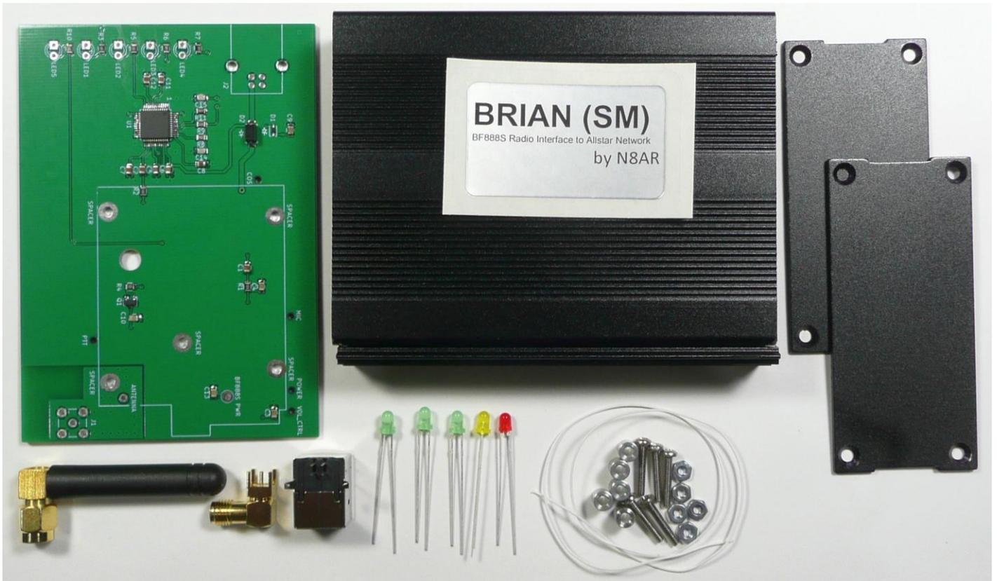
Figure 3: BRIAN (SM) Kit (BF888S Radio and USB Cable not Shown)
