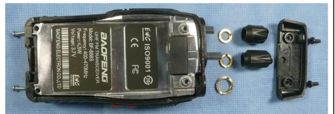
Remove the cast chassis and PCB by lifting the casting out of the plastic enclosure at the end which was held by the Torx screws. Position the two pieces as shown and unsolder the two speaker leads at the PCB. Recycle the speaker/plastic enclosure.
