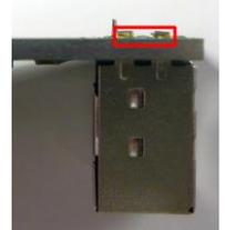
Insert the green LED with the formed leads into the board and position it as shown in the photos to the right. Note that the largest diameter part of the LED body is touching the PC board. Solder it in place and trim any excess lead length.
