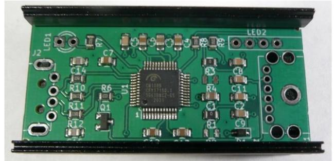
Attach the USB/LED end cap to one of the case halves using two end cap mounting screws. Place the USB connector in position on the PCB. Press the connector firmly to ensure it contacts the PCB then slide the PCB and connector into the case with the USB connector protruding about 1/8 inch through the USB connector slot in the end cap.
