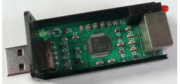
Place the other extrusion half in position on top of the bottom extrusion and fasten it to the USB end cap using two screws. Use care when installing the screws to avoid cross-threading them. The holes are tapped so the screws should turn easily.
