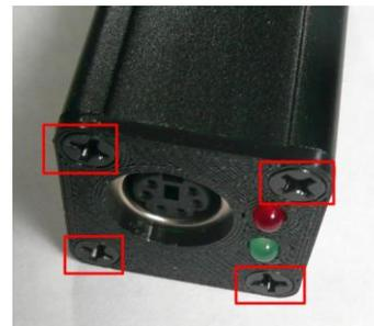
Clean the recessed area on the top of the case with isopropyl alcohol. Let dry and then apply the "DINAH" label in the recessed area in the top of the case. Ensure the label is oriented correctly so that COMMS, PTT and COS lettering on the label agree with the location of the LEDs at each end.
