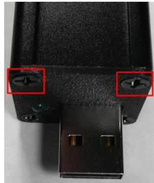
Attach the DIN end cap using four black flat head screws.
