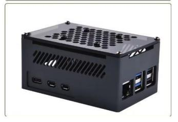
Unbox your Raspberry Pi5. Install two 11mm brass spacers from the SHARI kit, 4 short brass spacers and 2 knurled threaded fasteners (from the 52Pi/Pi5 case parts) as shown in the two photographs. Only tighten finger tight at this time.
