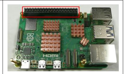
Mount the SHARI PiHat Mod2 PC board onto the GPIO connector pins and the two 11 mm brass standoffs. Install knurled fasteners onto the brass standoffs (shown in red boxes). Shift the positions of the two PC boards so that the GPIO connector pins are approximately centered in the PCB holes and tighten all mounting hardware.
