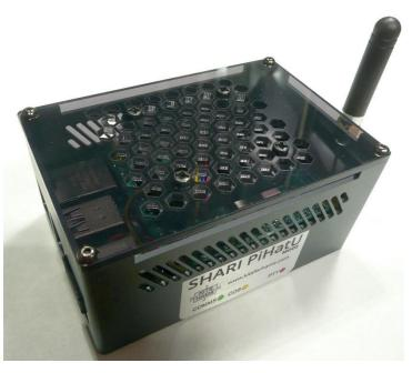
Unlike our other SHARI products that use an SMA connector soldered to the PC board, a coax cable with an SMA connector on one end and a U.FL (IPEX) male connector on the other is used to route the RF signal to the antenna. This simplifies construction and permits the antenna location to be easily changed by the builder.
