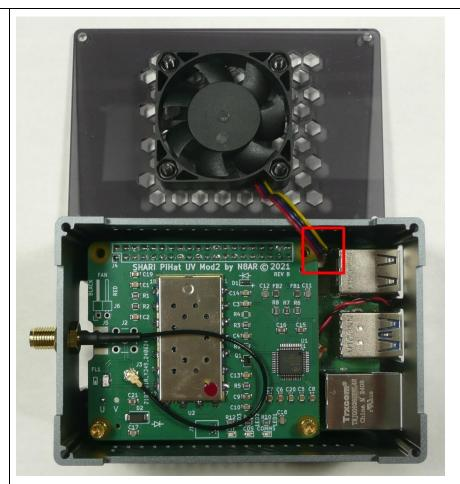
Install the top cover using the screws and Allen wrench provided with the 52Pi/Pi5 case.
