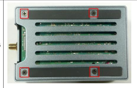
Route the coax cable with SMA connector as shown. Place the star washer onto the SMA connector with its tangs pointing toward the case. Thread a nut onto the SMA connector and tighten.
