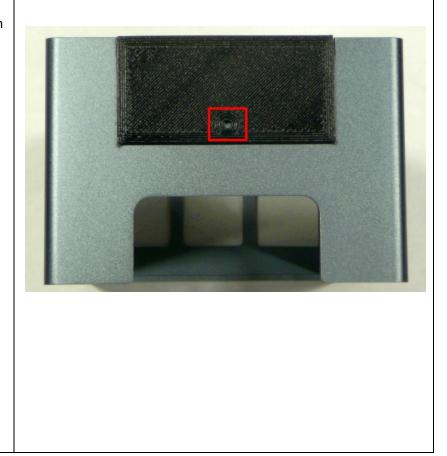
Drill a 0.25 inch hole. Remove a small amount of paint around the periphery of the outside of the hole to expose bare aluminum so that the serrated washer used with the SMA connector will contact bare aluminum.
