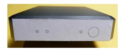
Drill three 1/16" diameter holes and one 9/32" diameter hole. The location of the 9/32" hole is the most critical. Use a good center punch. Start with a small drill and enlarge it gradually with larger drills or a step drill.
