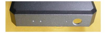
Locate the middle Neo case metal body. Drill a 1/8" hole centered on the #20 silkscreen (outlined in red in the photo) to route the internal USB cable from the Raspberry Pi to the SHARI PiHat
