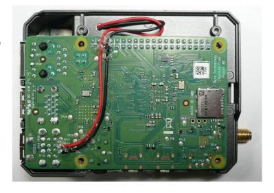
Remove the two screws holding the PiHat board and unplug it from the Pi. Remove the two screws temporarily holding the Pi. Raise the Pi and insert the Silicon thermal pad on the CPU. Place the Pi back in position, place the Neo plastic case over it and secure using four screws. Install the four rubber footings in the plastic cover.
