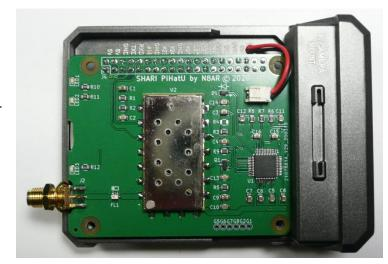
On the Raspberry Pi side of the assembly route the internal USB cable as shown in the photo. Solder the red wire to TP10 of the Pi and the black wire to TP6. Route the red and black wires **between** the GPIO connector pins as shown. Do not route them over the top of the pins as they may be pushed into the pins by the bottom cover risking the possibility of piercing the wire insulation. Fasten the cable in place using hot glue as shown.
