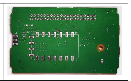
In this task, you will solder the SA818 radio module to the PC board in the U1 location. You will solder 18 castellated holes on the module edges to the pads on the PCB. If you have never soldered castellated holes before, please go to <a href="https://learn.sparkfun.com/tutorials/how-to-solder-castellated-mounting-holes/all">https://learn.sparkfun.com/tutorials/holes/all</a>
