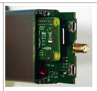
Install the two SHARI PiZero labels and the antenna as shown.
