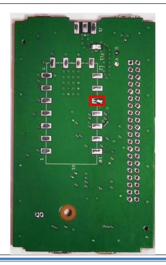
Use the following procedure to solder the module. Observe that there are castellated holes on only one end of the SA818 module. Be sure to orient the module so the castellated holes on the module align with all the PC pads on the board.
