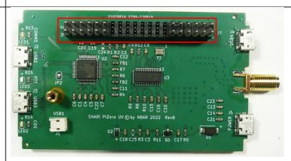
Place the PiZero 2W in position on the two 12 pin male pin headers and the 7mm standoff. Install a 2.5 mm screw into the 7mm standoff (yellow rectangle). Center the screw in the hole and tighten.
