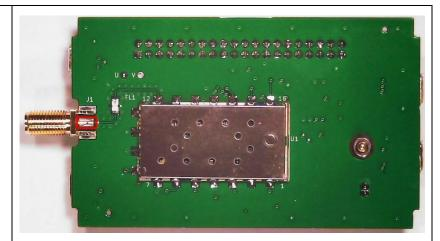
Place the 3D printed end cap over the SMA connector and two microB USB jacks to verify the proper location and alignment of the SMA connector. Reheat the lightly soldered center pin solder connection and reposition the SMA connector as required.
