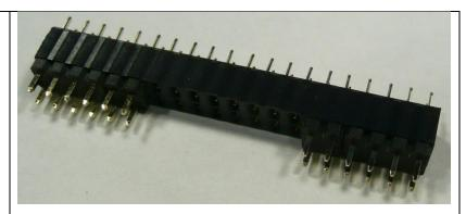
Place the 40 pin female header with 12 pin male pin headers in position on the SHARI PiZero motherboard as shown in the photo. Note that the female connector pins plug into holes in the SHARI PiZero motherboard.
