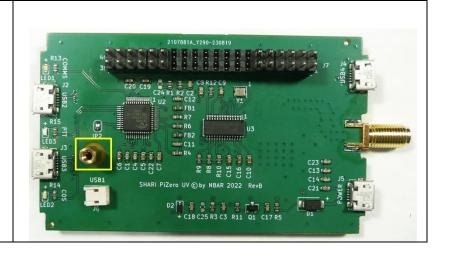
Next you will place the GPIO connector assembly in position. Note that it consists of a 40 pin female pin header with 12 pin male pin headers inserted at each end. (Note that each 12 pin male header is actually an 8 pin and a 4 pin header).
