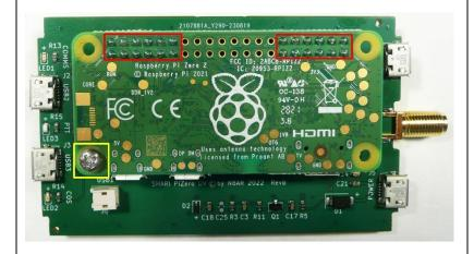
Ensure that the GPIO connector assembly is firmly seated (no gap) on the SHARI PiZero motherboard and solder 12 pins (2 rows of 6) at each end of the connector. (If you accidently solder more than 12 it is OK as there are no connections to these pads on the SHARI PiZero motherboard)
